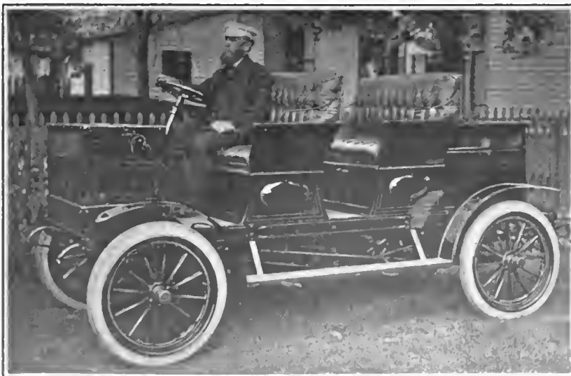
KEROSENE BURNING STEAM CAR BUILT BY GEORGE A. HENDERSON.
